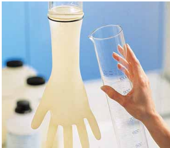
Water retention test
